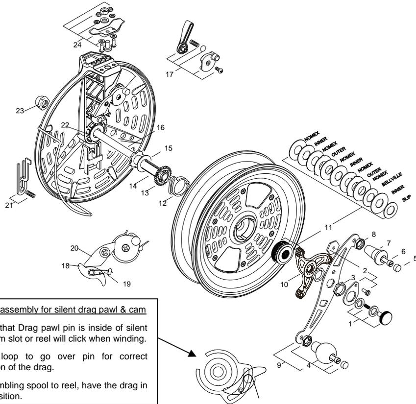
Correct assembly for silent drag pawl & cam
