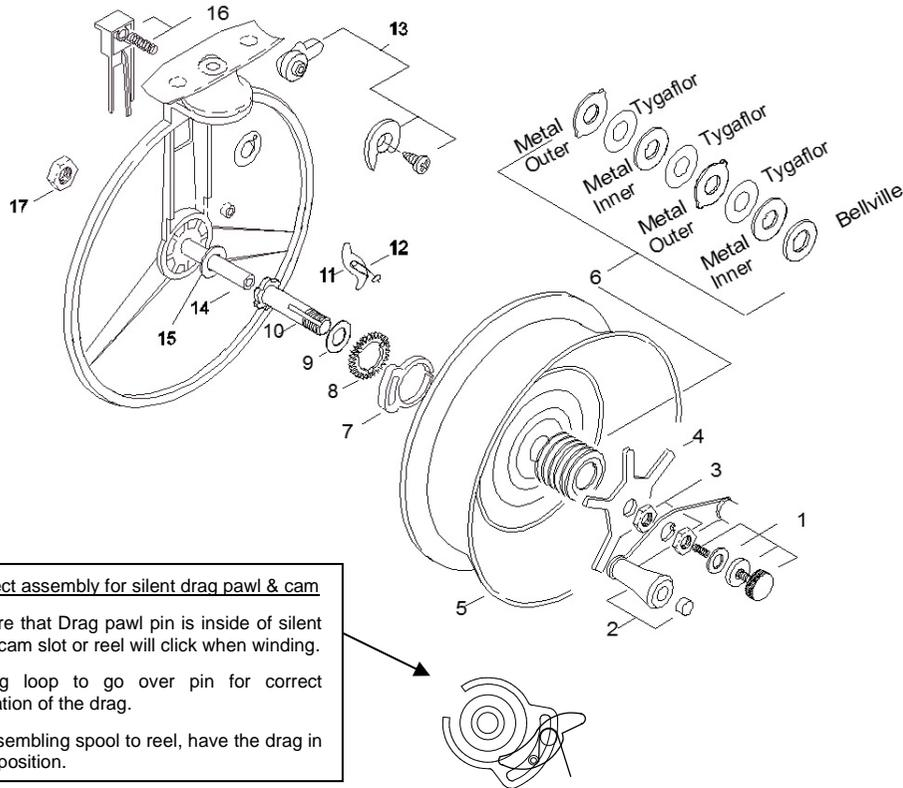
**Correct assembly for silent drag pawl & cam**
